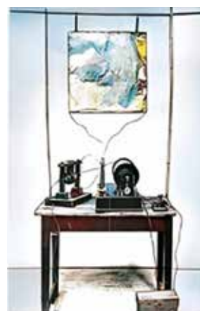
Marconi's original wireless with copper sheet aerial
